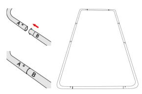
Please connnect tube A with tube B by pressing down the spring pin,until it is bounced back.
