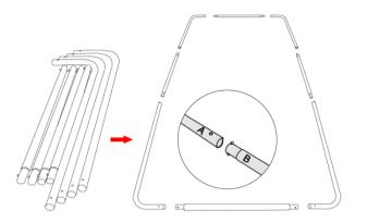
Each frame is combined by 4pcs straight tubes-A and 4pcs curved stubes-B. (As picture).
