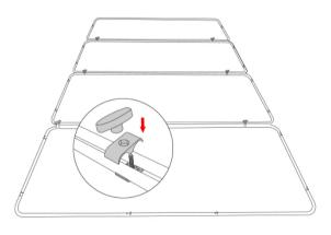
Use hinge clips to connect two frames.
